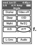
**2.** To turn the attenuation feature off, tap the **ATT** on the remote control unit again.
